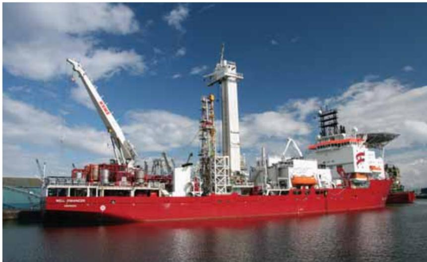
the Well Enhancer provides a larger bore intervention system which allows access to a greater number of subsea wells. It features a 150 ton multipurpose tower capable of deploying wireline, slickline and coiled tubing tools - the addition of the CT system has expanded the vessel's already impressive workscope capabilities. The vessel also features kill pumps, an intervention lubricator control system and an active heave compensated main winch.
